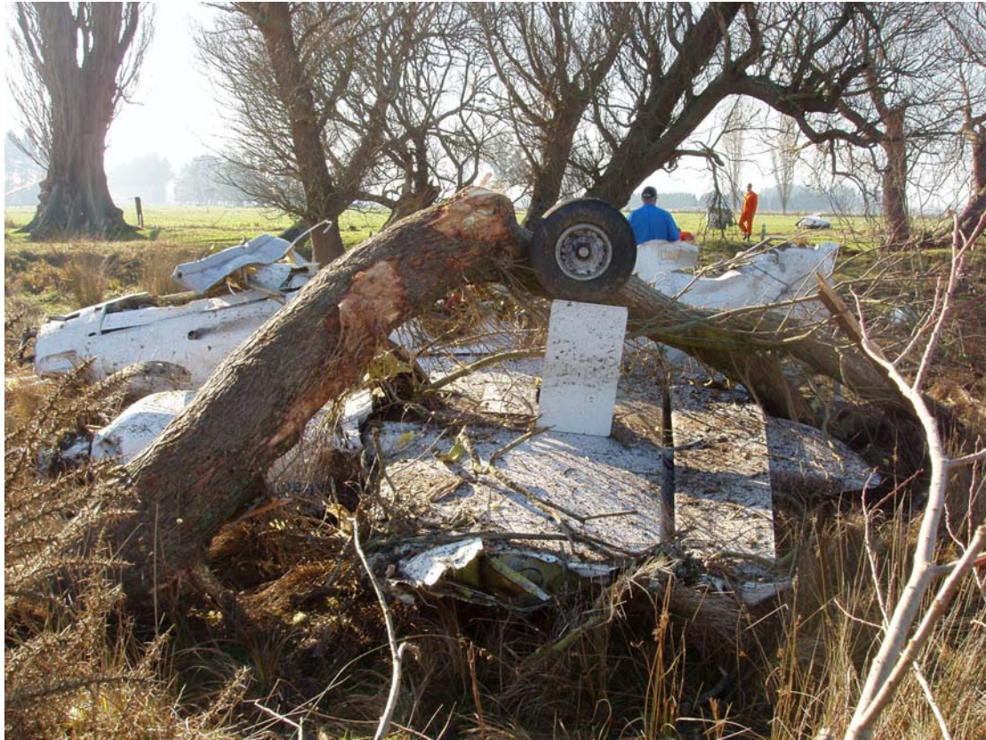
This Chieftain multi engine aircraft hit trees while on an instrument approach to Christchurch International Airport killing eight people and seriously injuring two (2003).
