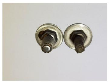
The screen filter on the left of the photo is the new design screen filter, which has a solid metal disc at the aft end of the screen filter.
