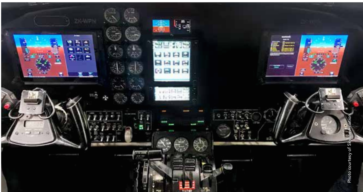
// Skyline Aviation in Hawkes Bay carried out an electrical load analysis when it upgraded its King Air B200 with a Garmin G600 TXI Avionics suite.
