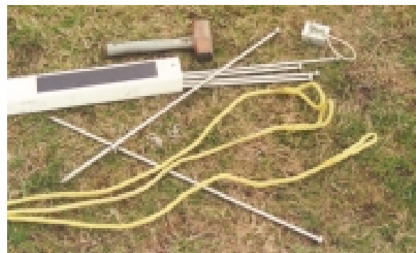
A lightweight set of pickets utilising stainless steel rods and twisted shackles stored in a plastic (downpipe) tube.
