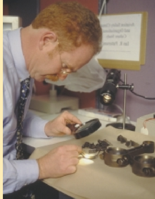
A CAA Accident Investigator inspects a crankshaft bearing from a failed engine
