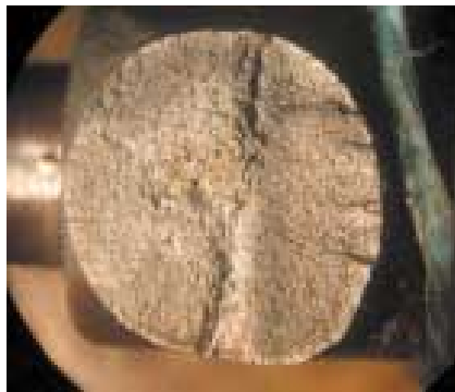
A cross-section of the failed Pitts tailwheel fork.
