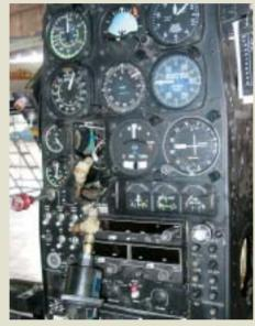
The accident helicopter's instrument panel, showing the broken torque and oil pressure gauge supply line fittings. Photograph courtesy of TAIC.
