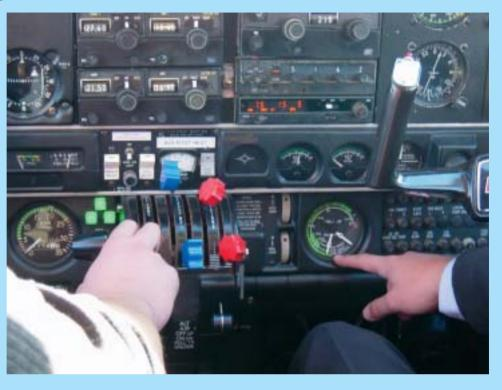
thinking that they were in fact the fuel pumps, the consequences of which did not become apparent until the loss of manifold pressure was noted. In the meantime, the student had also turned the lefthand engine magneto switches off confusing them with the landing light switches as the last item on the checklist. (The magneto switches are located directly above the landing light switches and have a cover over them to prevent them being inadvertently selected, which the student lifted.)
