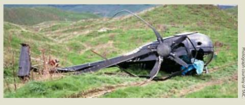
In its accident investigation report, the Transport Accident Investigation Commission (TAIC) identified that the helicopter's engine had failed due to oil starvation following the fracture of a nylon tee fitting in the engine torque gauge oil pressure feed line system.
