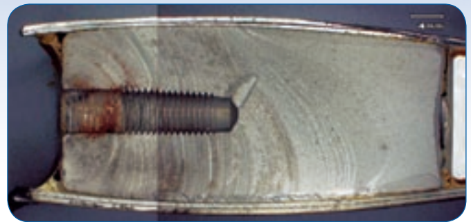
Fracture surface of an R22 blade root, showing fatigue cracking in the root fitting. Note: Growth of fatigue is obscured by external skin and doubler.
