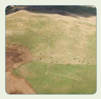
From the photograph, it can be seen that this mast is very hard to see even in good weather. The ground at the site is approximately 300 feet **amsl** (100 metres), and the mast height is just under 200 feet **agl** (60 metres). If the pilot had been at 500 feet amsl over the sea, then the turn inland would indeed have been a hazardous manoeuvre. Now there's a lesson.
