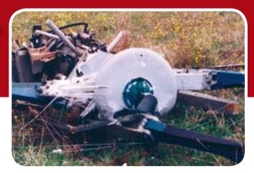
This gave one blade unlimited freedom in the plane of rotation – with a major shift in the centre of gravity of the rotor system. The forces resulting from the imbalance were immense, as in all three cases the entire main rotor system **and transmission** were torn bodily from the airframe. Freeze-frame the imagination there if you like.
