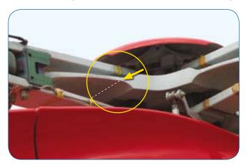
The line of cross-section change was the line of the impact failures
