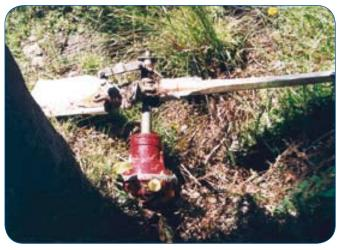
The result of the strike was the departure of the tail rotor and 90-degree gearbox from the airframe.
