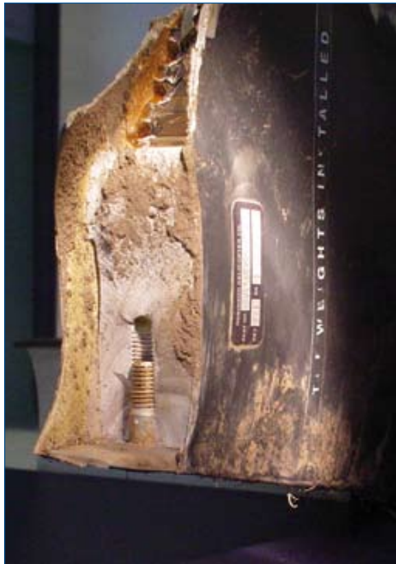
This is a Robinson R22 main rotor blade that failed as a result of metal fatigue. The fatigue striations are clearly evident on the fracture surface. This can occur if the blade is used beyond its design life, or subjected to loads greater than those anticipated by the manufacturer, or a combination of both.
