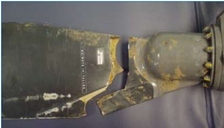
This is a Robinson R22 main rotor blade that failed as a result of metal fatigue. The fatigue striations are clearly evident on the fracture surface. This can occur if the blade is used beyond its design life, or subjected to loads greater than those anticipated by the manufacturer, or a combination of both.
