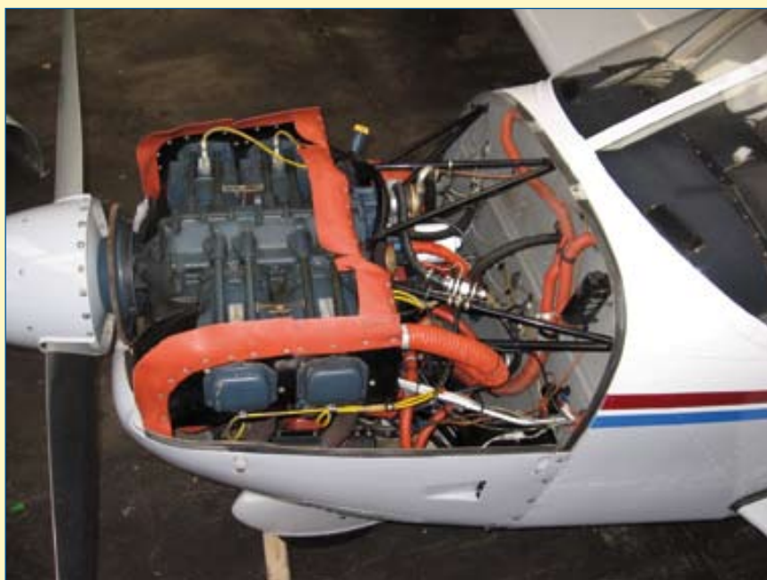
Correctly installed baffle seals in good condition.
