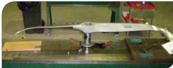
A bent propeller that can be repaired.
