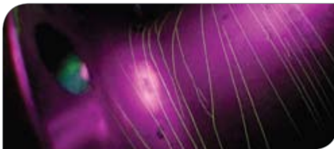
Cracking of the crankshaft after impact damage, shown up by fluorescent light during magnetic particle crack testing.
