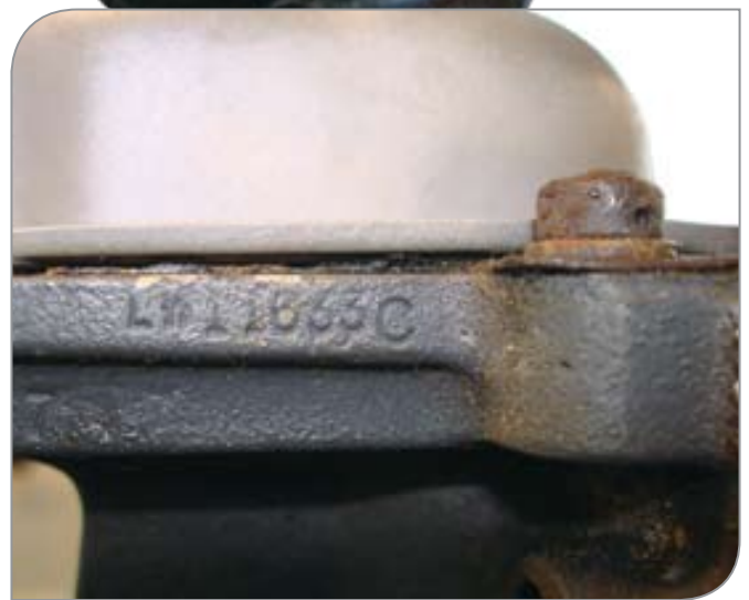
Chrome plated cylinders should be colour coded orange and have "C" added to the part number.
