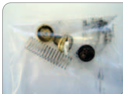
The other parts of the G-switch. The layer of black powder is evident on the ball. The black spot in the centre of the end cap on the left is fretting.
