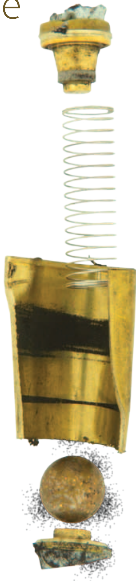
The other parts of the G-switch. The layer of black powder is evident on the ball. The black spot in the centre of the end cap on the left is fretting.
