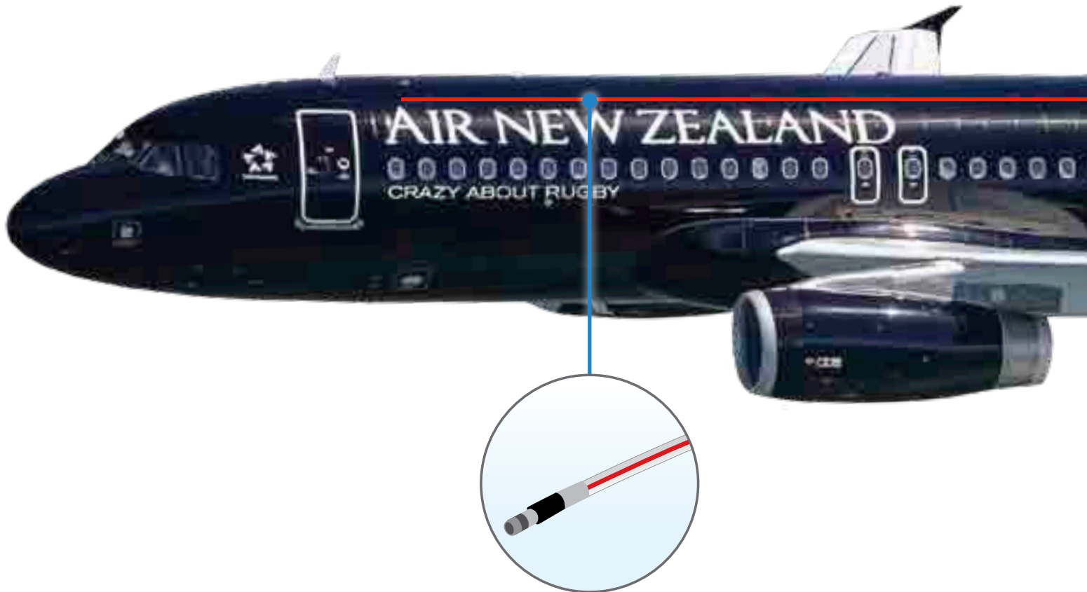
Leaky Line Antenna
