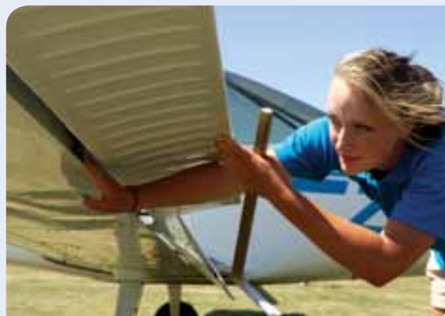
Beware the finger traps some ailerons can pose. Keep a firm grip on the trailing edge while checking pushrods, locknuts and the like, as demonstrated by Nari Casley.
