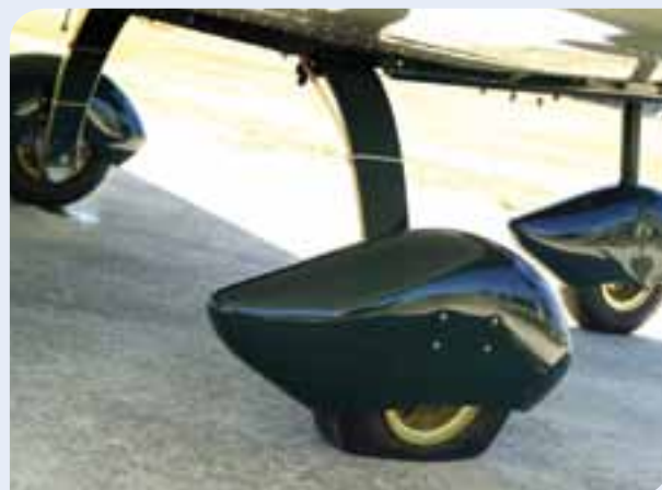
The flat tyre might be obvious, but what about that stain on the ground by the left main wheel?
