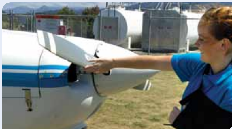
Keep clear of the propeller arc, as shown by Nicole Patterson, and take care when checking the leading edge – there can be sharp-edged nicks present.
