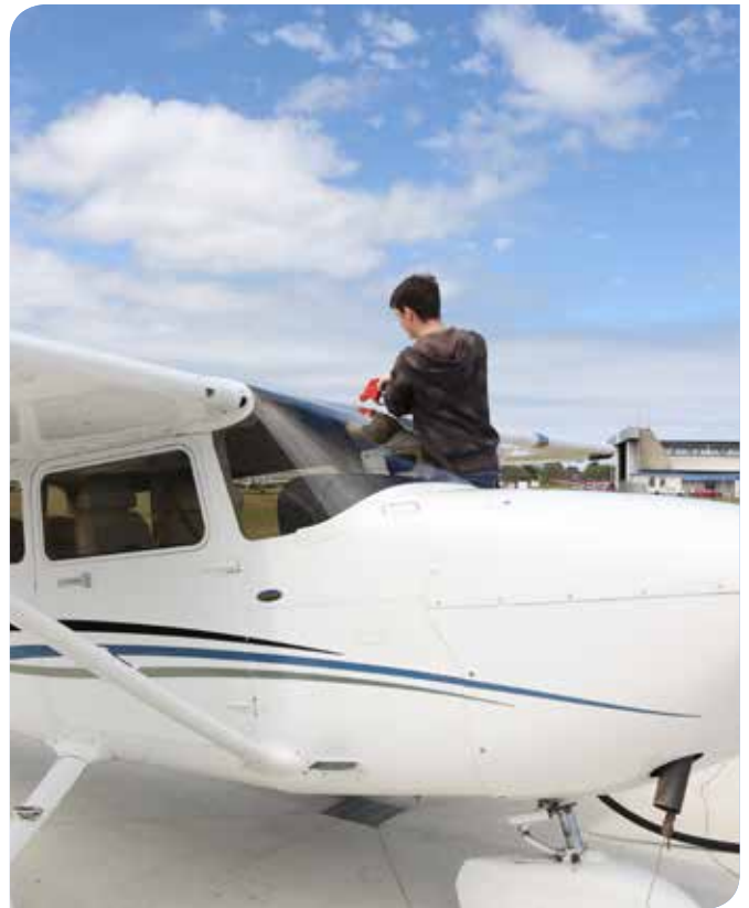
Benjamin says that topping up fuel tanks after landing will minimise the chance of condensation forming if the aircraft is going to be left for some time. It will also add mass to the aircraft providing stability in wind.
