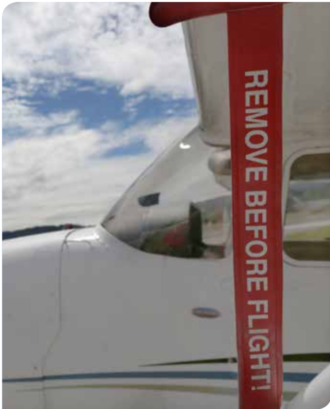
Accurate airspeed indication is vital, so keep the pitot tube covered to keep bugs out when not flying.
