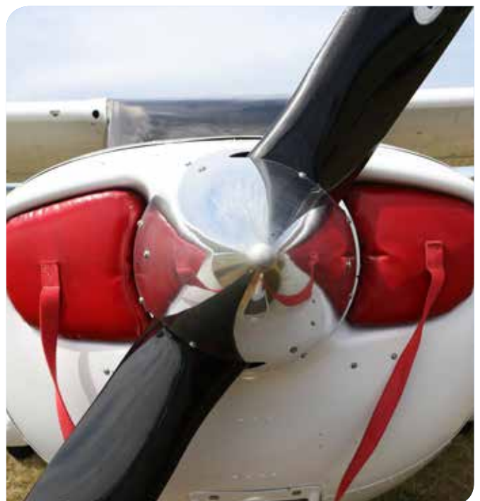
Engine blanks prevent nesting birds and windblown dust and dirt damaging the engine.
