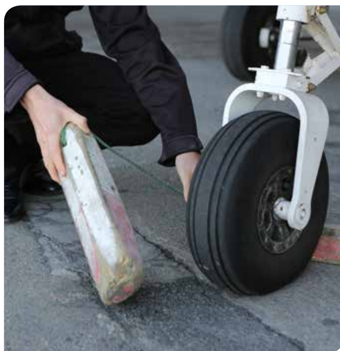
Don't rely purely on your aircraft's park brakes. Chocking the wheels will add security – and peace of mind.
