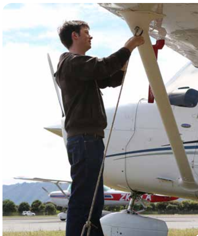
Benjamin Petersen of Kapiti Aero Club picketing the aircraft. That will stop the aircraft being moved around, or even flipped over, by a buffeting wind.
