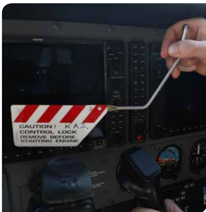
Control locks prevent damage from wind gusts.
