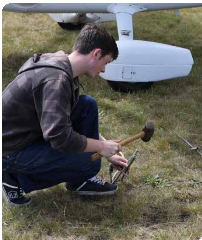
Benjamin Petersen of Kapiti Aero Club picketing the aircraft. That will stop the aircraft being moved around, or even flipped over, by a buffeting wind.
