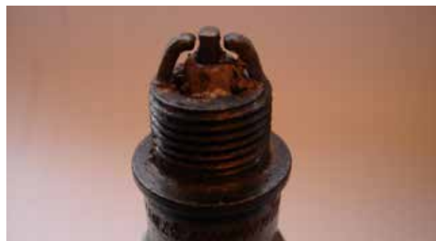
// An example of a fouled spark plug, also from a Cessna 152. See GA defect next page >>
