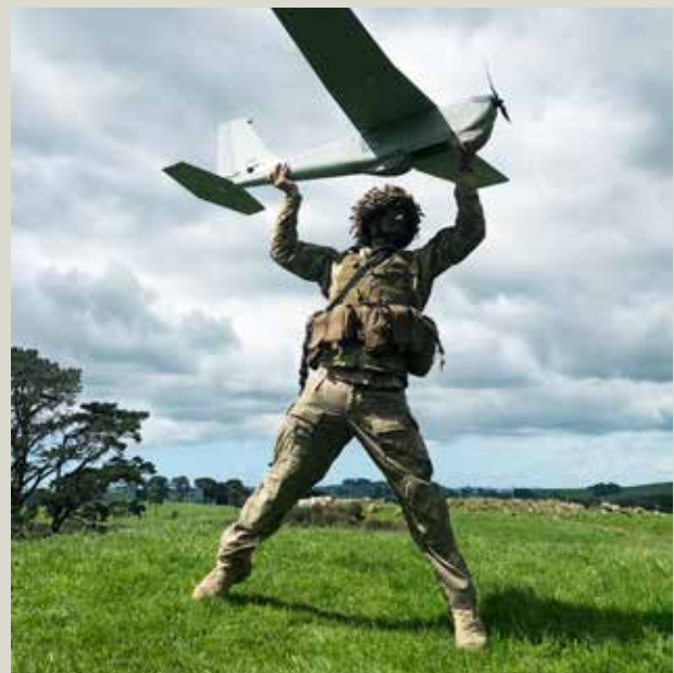
// The Puma UAS being launched by hand as part of a military training exercise.
