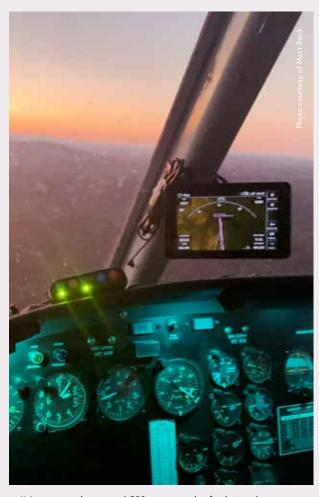
$\ensuremath{/\!/}$  A permanently mounted GPS – an example of a design change.
