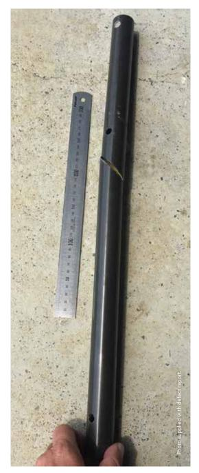
"Continuing airworthiness notice 27-014 was issued in February 2020 to "bring attention to a defect reported to the CAA of finding a severely cracked pilot to co-pilot tail rotor torque tube on a Hughes 369FF".
